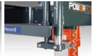
Automatic gate lock on elevation
